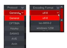
The "general" POS protocol and additional encoding options make the NVR compatible with most POS brands. The POS is now easier to configure, and it reduces technical support requests regarding the POS configuration.
