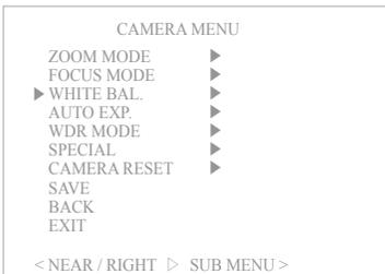
White balance setting is a function revising color temperature to resolve the problem that screen's colors change by the color temperature's difference according to time.
