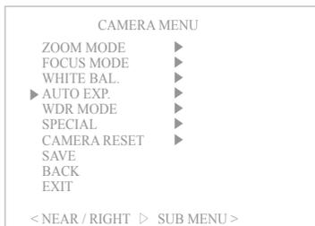
AE setting is a function adjusting shutter speed according to subject's brightness to get standard amount of exposed light.
