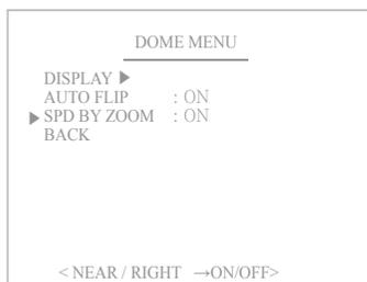
When this function is ON, the pan/tilt speed is inversely adjusted to the zoom ratio.
