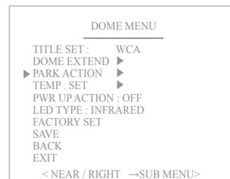
This function enables to locate the camera to specific position automatically if operator doesn't operate the controller for a while.
