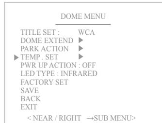
It shows you the current temperature and you can also set the value manually. The compulsory Fan & Heater operation is a useful function to remove humidity.
