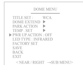
When this function is ON, the camera memorize the latest action and restore it from sudden power failure.
