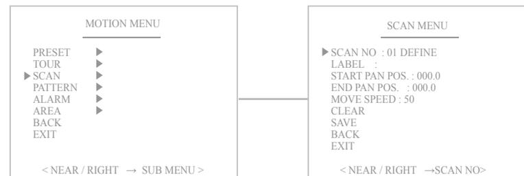
The Scan function means that the camera keeps panning between two programmed pan positions. It is also adjusts the moving speed(1~63 step). Maximum 4 Scan functions are toured in order.
