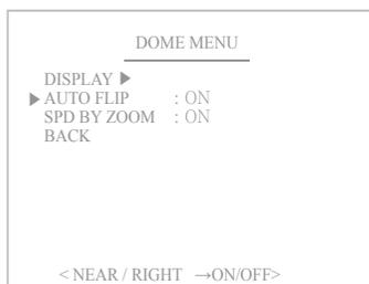
You can observe the moving object without reversing of the screen, by using this AUTO FLIP function. ON: If this function is set to ON, camera will be automatically flipped in tilt 90°
