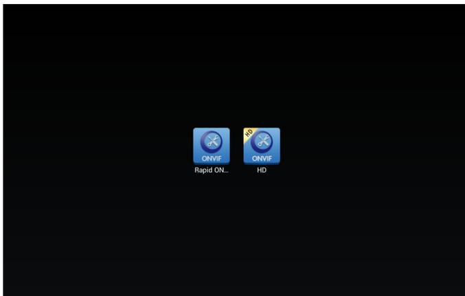
If you select ONVIF Rapid mode, the meter automatically scan different network segments for ONVIF cameras. It lists the camera name and IP address on the Device List. Tester can auto login camera and display camera image .
