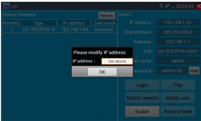
For other operations need login activated camera, when login, select the camera at the left “online detection”, and input username and password to login.
