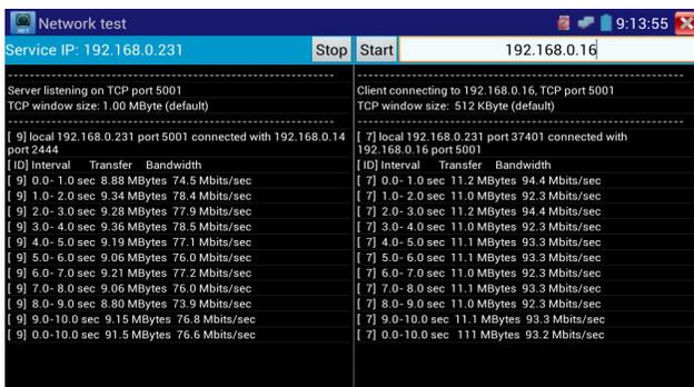
Network bandwidth testing can also be tested with a computer using compatible network bandwidth testing software. Install network bandwidth testing software on a computer, as a test Client or Server, to do the mutual testing with the tester. If use computer as the server, the computer IP address is :192.168.0.89
