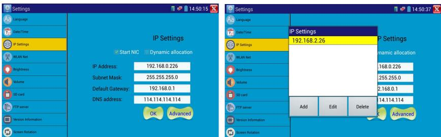
After setting an advanced IP address (refer to the photos above), the unit can test two network segments (192.168.0.0) and (192.168.1.0)
