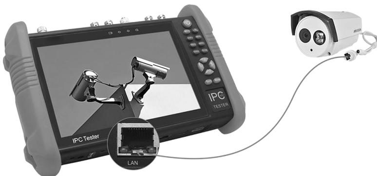
**Note:** 1) If the IP camera requires PoE power, then connect the IP camera to the IP tester's LAN port. The tester will supply PoE Power for the IP camera. Click on the icon labeled POE to turn the PoE Power off or on.
