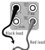
b. select  $\tilde{A}$ , enter the AC current measurement, manually select the range
