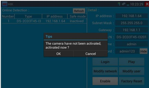
1. **Hikvision activation:** When connect the unactivated Hikvision camera to the tester, it will auto identify and display “Unactivate” at safety mode. Select needed activate the camera, click bottom right corner button “Enable”, pop-up “the camera is not activate, activate now”?
