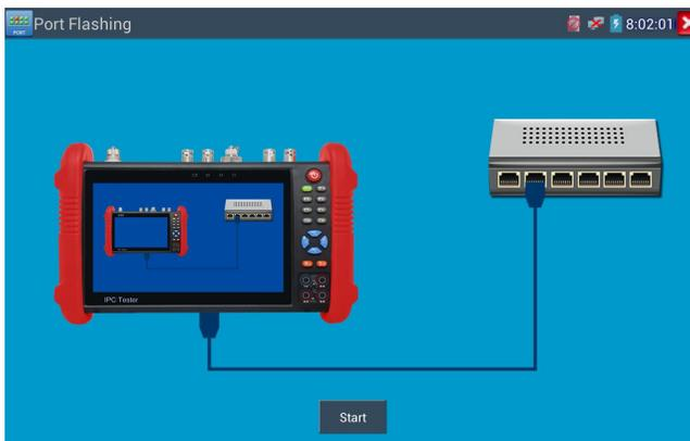
If the tester and PoE switch are connected well, the LAN port of POE switch flash at special frequency,
