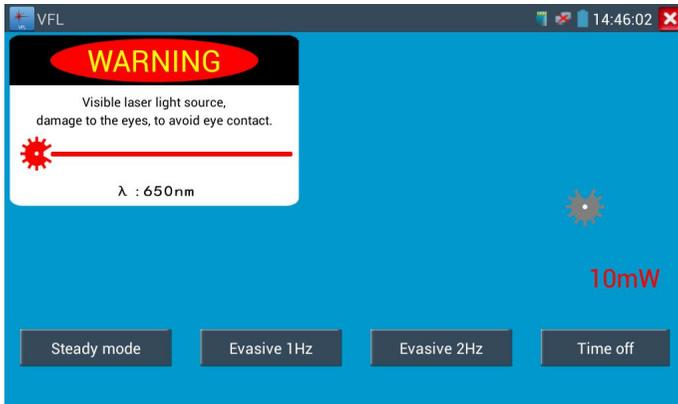
VFL four status can select——“Steady mode”, “Evasive 1Hz”, “Evasive 2Hz”and“Time off”. Click button “Steady mode” to enter steady status, click button “Evasive 1Hz” and “Evasive 2Hz, to enter pulse mode, click button “Time off”, VFL is turned off. Timed turn off can select (5 mins, 10 mins, 30 mins, 60 mins and 120 mins).
