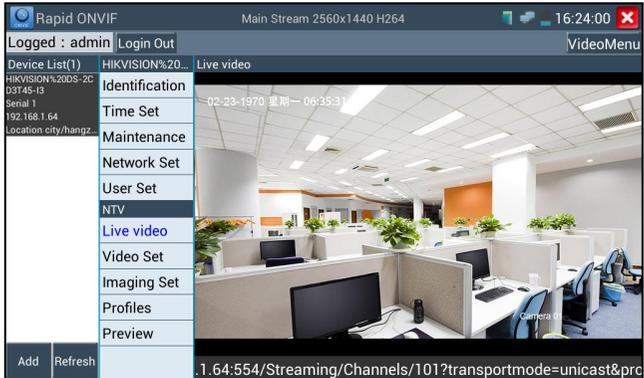
If your IP camera does not appear after scanning the network, you can manually add an IP camera by clicking on the “Add” button on the bottom left. The URL address should be identical to the ONVIF camera service address. (With your camera’s IP address entered into the URL). Click OK to add the manually entered camera and then click the “Refresh” button.
