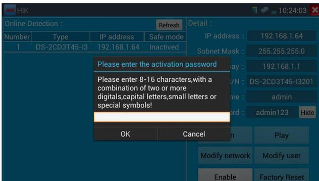
**2. Input password:** Input new password, tap “ok” to activate
