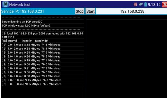
b). **Start send packet test:** Using the other IP tester, type in the Server's IP address at the top right corner of the screen. This app is used to send packets for network speed testing. Click the “Start” button to send the packets and start testing.
