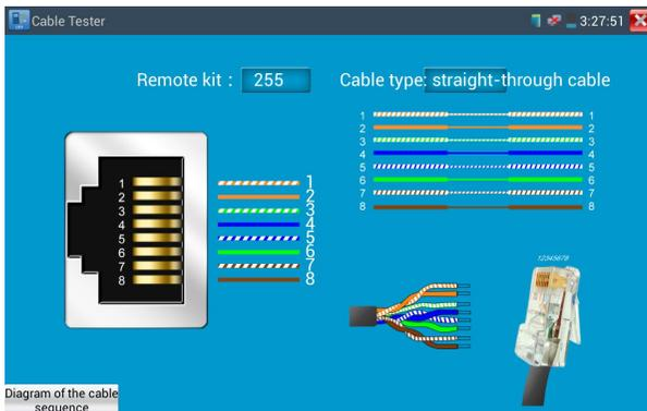
Test LAN cable or telephone cable.
