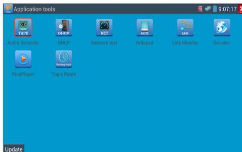
**Audio Record:** Connect an audio device to the IP tester's audio input port. Click the
