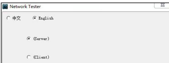
Tester as Client, tester's IP address is:192.168.0.230. The Server and the Client are at the same network segment, but with different IP address. Input Server's IP address 192.168.0.89 in the tester and click "Start" to test network bandwidth.
