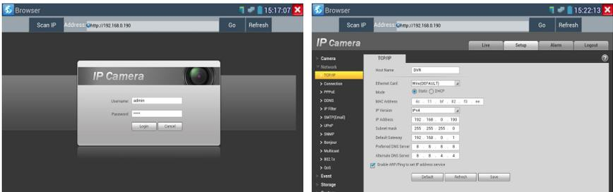
The IP camera and IP tester be on the same network segment for the browser to interface with the camera. If they are not in the same segment, click the button
