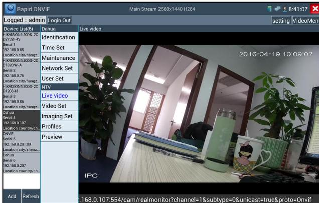
**Live Video:** Click “Live Video” to view the live video feed from the IP camera. To make the image full screen, double tap on the video. Stretch two fingers outward or inward on the touch screen to zoom the image in or out.
