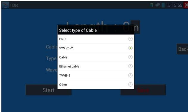
3. Click “+” or “-” to adjust wave speed, while display length is the same with the actual Length, click “Save” to save calibration data. It can be used for the same cable testing next time.
