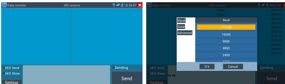
Click “Setting” to choose the baud rate of RS485; it must be the same as the DVR or the Control keyboard .The DVR or Control keyboard send the code to the tester, if it can be read, the protocol will
