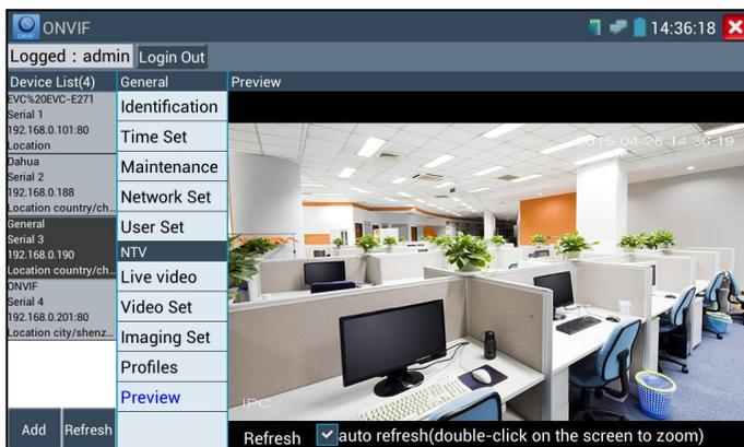
**Network setting:** Click “Network Set” to change the IP address settings. Note: Some cameras are not fully ONVIF compliant and cannot support changing their IP address, so there is no change after saving.
